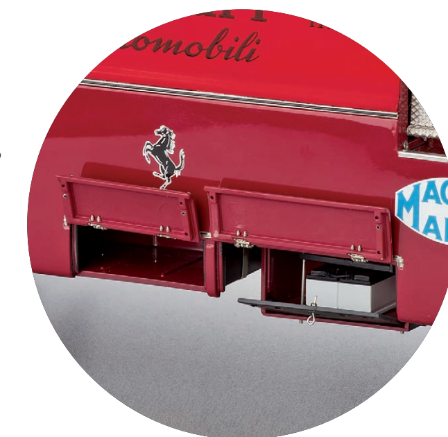
Finely-hinged flaps that enable access to the storage space and battery.
