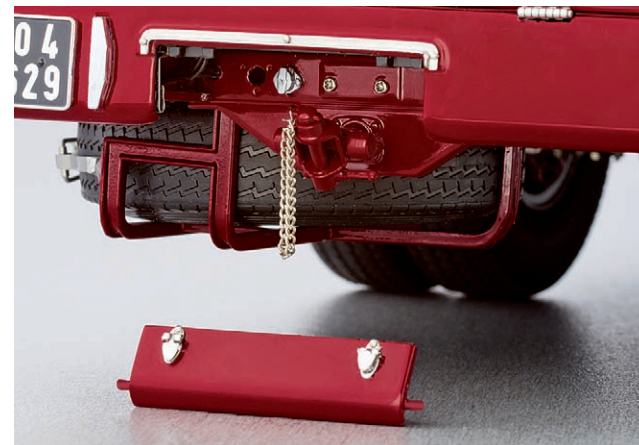
Behind the removable cover is a flanged towing hitch.
