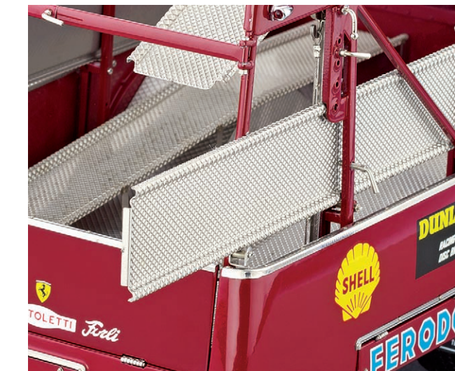
The ramps can be shelved sidewise and held in place with toggle screws.
