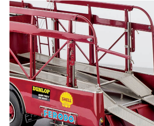
The highly-detailed and functional auto hoist can be moved up and down manually. The rails are made of authentic checker-pattern metal plate.
